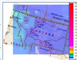
Fig. 4. Tinting: \text{Hg}_{\text{TOT}} deposition <10 \mu\text{g m}^{-2} \text{y}^{-1} (EPRI TEAM model); base map: Montana waters with fish levels >0.3 \text{ ppm Hg} (icons).
