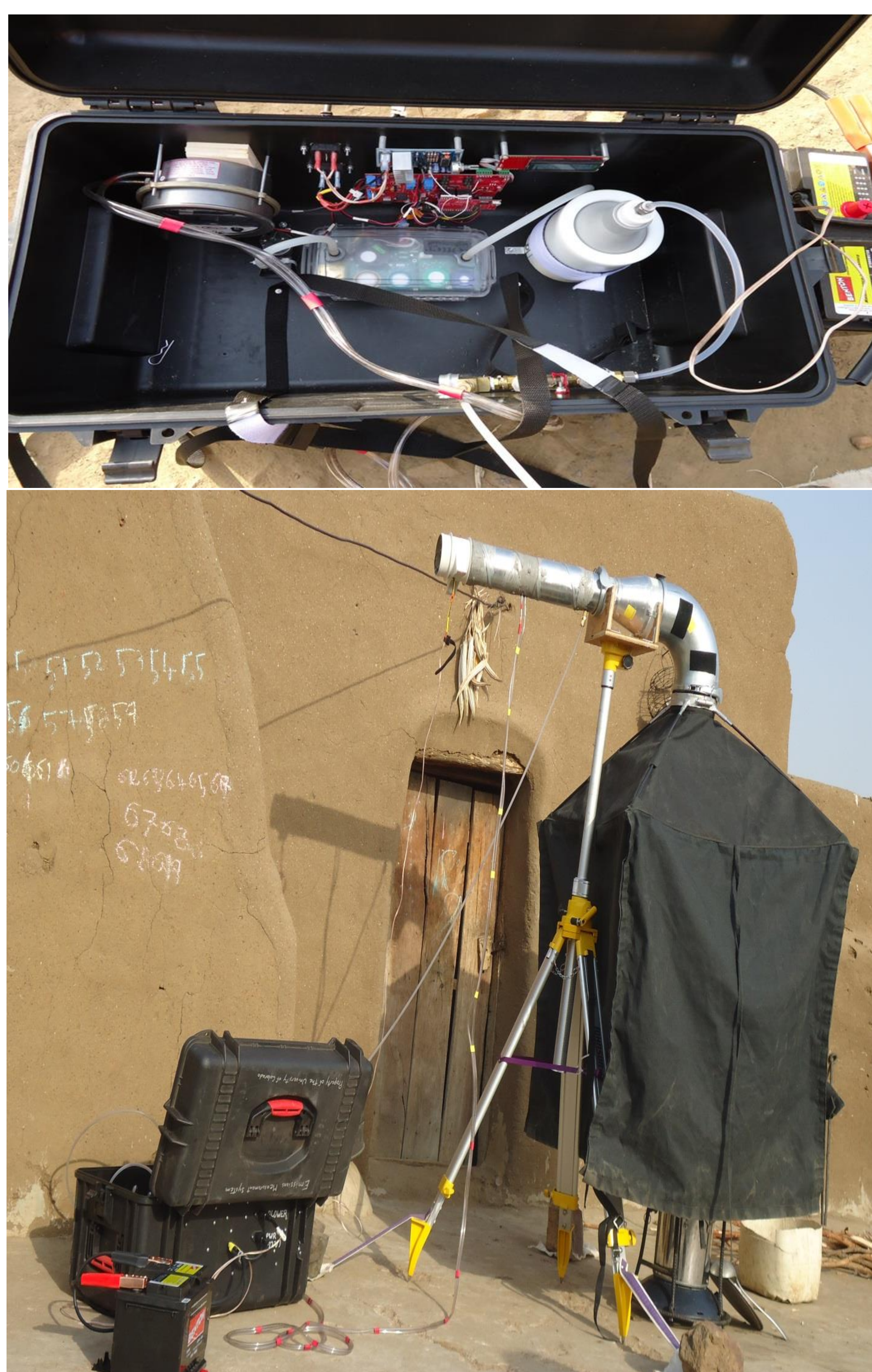
Figure 1. The Portable Emissions Monitoring System (PEMS) set-up in the field in Ghana and inside the emission pod box with sensors.
